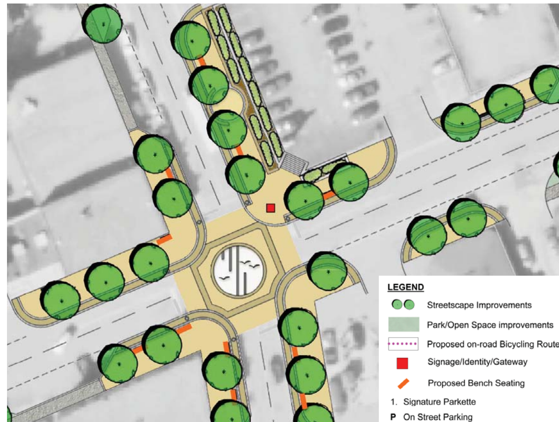
Figure 19: Detail Plan - Intersection Improvements
